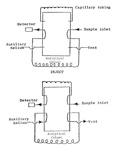
BACKFLUSH FIG. A1.1 Schematic of Flow System Utilizing an 8-Port Sliding Plate Valve with a Single Column
