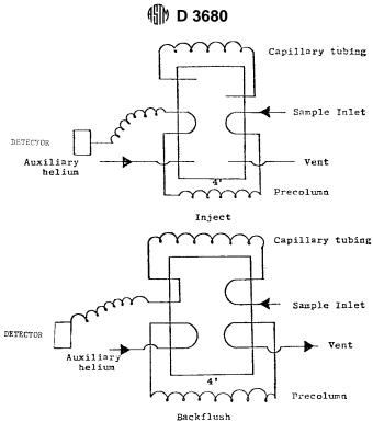
FIG. A1.2 Schematic of Flow System Utilizing an 8-Port Sliding Plate Valve with Two Columns
