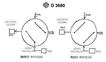
NOTE 1—At a predetermined time, after the monomer peak has passed through the precolumn, the valve is activated to flush the solvent out the injection
