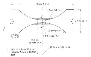
Material 0.2 mm (0.007 in.) spring steel. All springs use same 107-mm (4-3/16 in.) R base arc.
