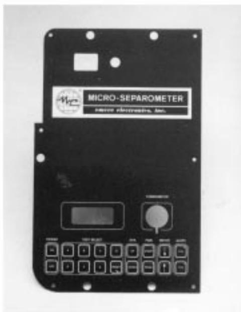
FIG. 1 Micro-Separator Mark V Deluxe and Control Panel
