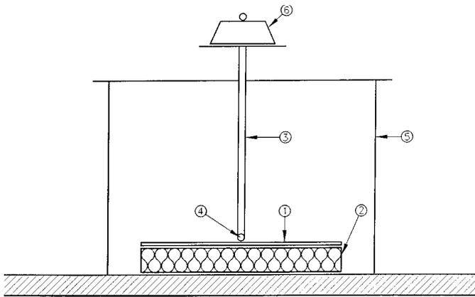
NOTE 1—membrane test specimen; 2—insulation substrate; 3—movable rod; 4—ball bearing; 5—framework supporting the moveable rod and load; and 6—load.
