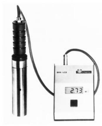
FIG. 2 Conductivity Meter
