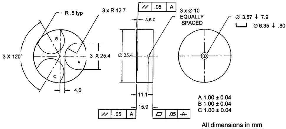
FIG. 7 Gage Block Used to Calibrate Displacement Transducer
