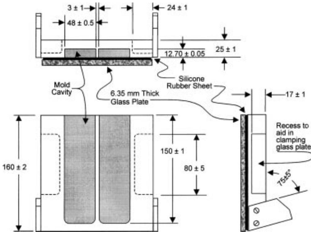
FIG. 5 Dimensions for Fixture for Silicone Molds
