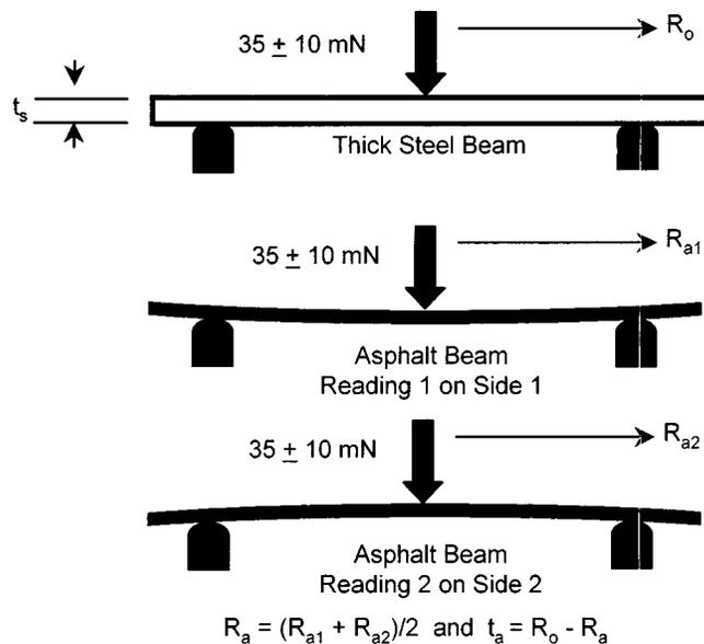
FIG. 8 Specimen Thickness Measured with Displacement Transducer
