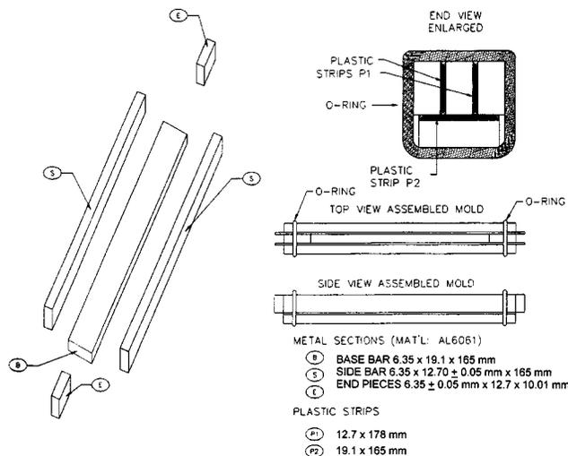
FIG. 4 Dimensions and Specifications for Aluminum Molds
