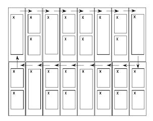
Note—"X" denotes specimen orientation. If multiple specimens are in a single holder, they do not need to be repositioned within the holder. FIG. 1 Specimen or Specimen Holder Repositioning for a Xenon-Arc Device With a Planar Exposure Area caused by stain or deposit, run referee tests in at least one other laboratory that can meet the water quality requirements described in 8.4.
