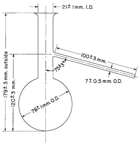
FIG. 1 Distillation Flask
