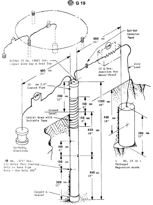
FIG. 1 Three Specimens in a Circle with a Common Anode
