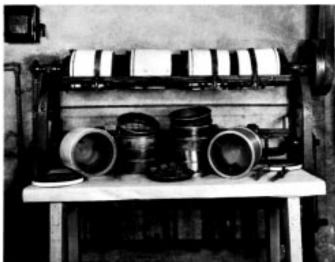
FIG. 1 Steel Frame Used in Jar Mill
